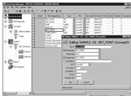
MX Change is integrated in the MELSOFT family as the "heart of automation". The software package consists of a Server and a Super Projekt Manager, other automation programs can be connected to. Since MX Change operates across a network, any variable once declared can be used by all other systems connected to the database.
